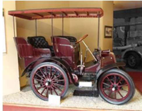
Royal car, 6 hp 2-cylinders 1527 cc fitted with a "mail phaeton" body
