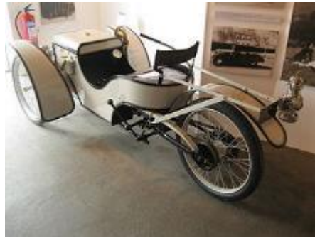
Rear view of Morgan Runabout showing swingarm rear suspension
